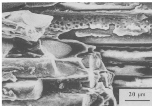
Figure 8 T orientation thermally cycled sample showing numerous voids at the fibre/matrix interface.
