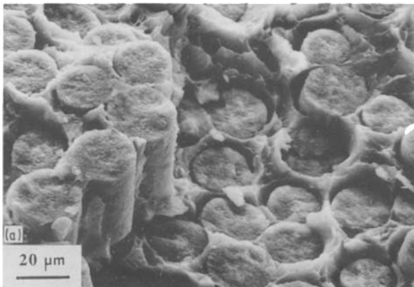
Figure 4 (a) Fractograph from L orientation tensile sample showing cliff, small amount of debonding and matrix ductility. (b) Fractograph from T orientation tensile sample showing predominantly fibre/matrix debonding.
